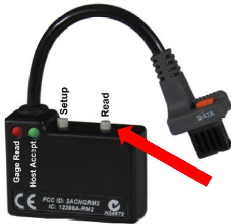
Mobile Module Buttons and LEDs
