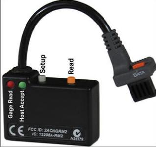
To set up a MobileCollect Mobile Module, you must put the Module into the Setup Mode and then send the current Module parameters to the setup Program.
