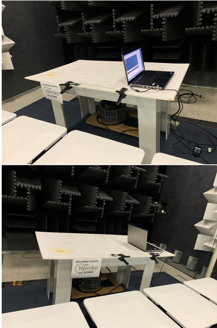
Figure 8.1-2: Clause 9.2 – Radio frequency electromagnetic field (2.7 GHz to 6GHz) setup photo
