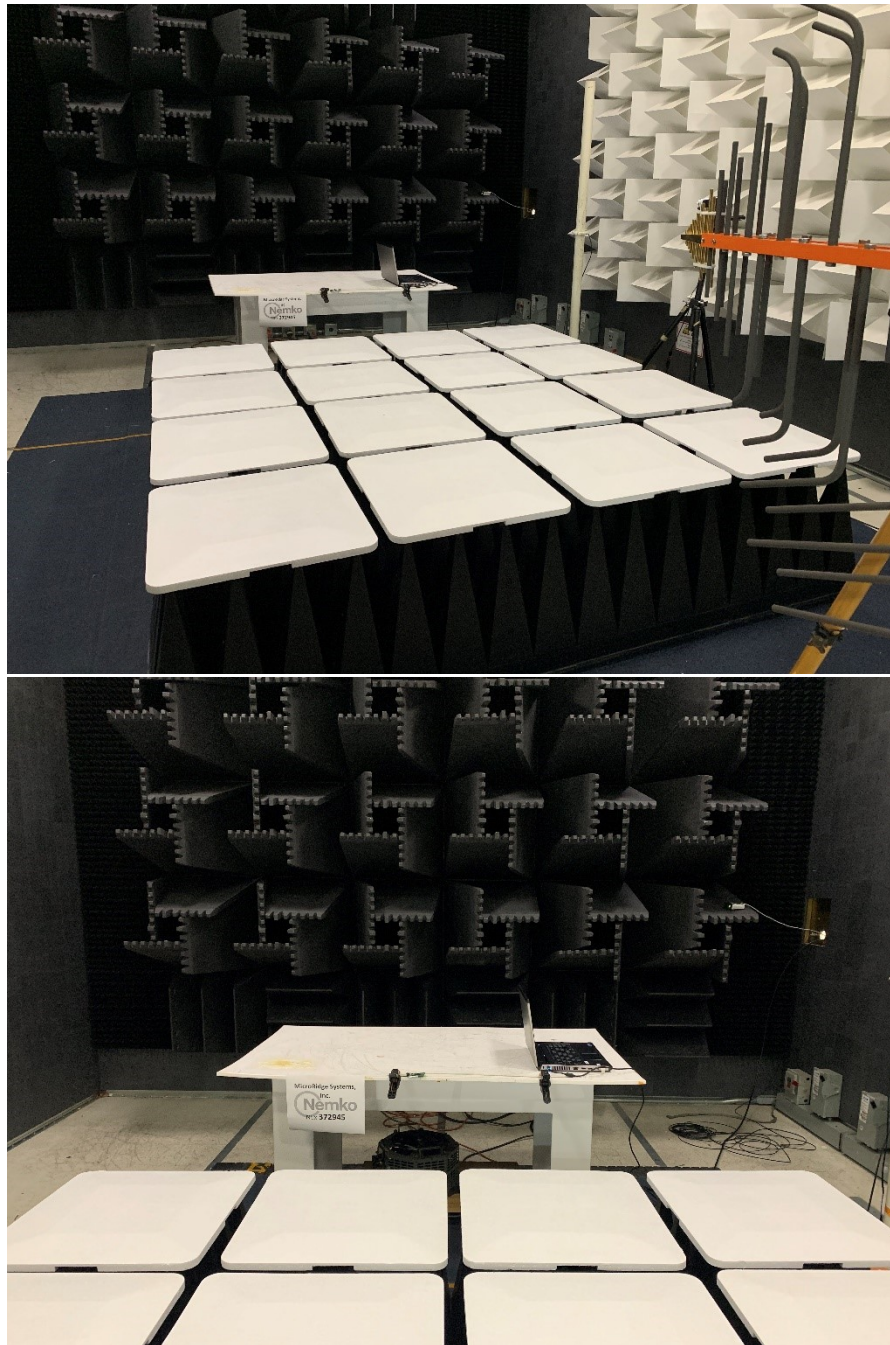
Figure 8.1-1: Clause 9.2 – Radio frequency electromagnetic field (2.7 GHz to 6GHz) setup photo
