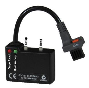
**Mobile Module Buttons and LEDs**
